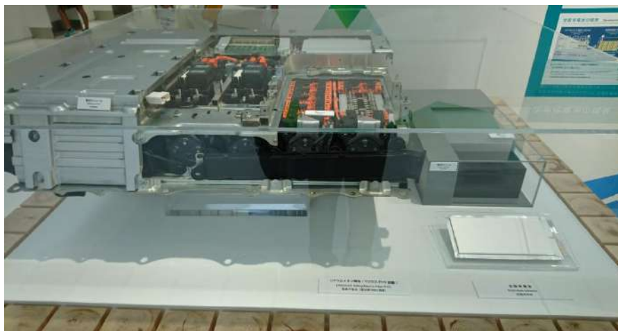
Figure 6. Toyota Motor: Lithium-Ion Battery (fitted in Prius PHV) vs. All-Solid-State Battery (Developed Product) — Sharp Difference in Pack Volume Between the Lithium-Ion Battery on the Left and the All-Solid-State Battery on the Right
